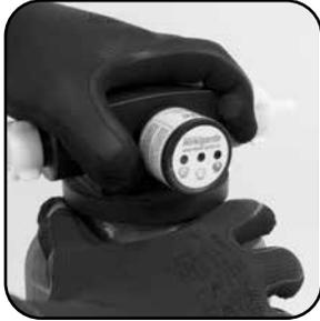
Release the water pressure from the cartridge and unscrew the connection fitting.
