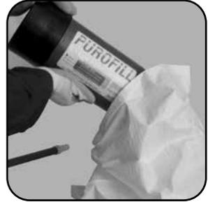
Empty the old mixed bed resin into a collecting bag and dispose it in the residual waste.
