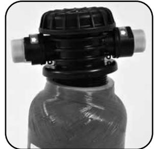
Screw the connection fitting hand-tight onto the cartridge. **Attention!! Do not tilt the connection fitting. This can damage the internal thread. Pay attention to the correct position of the o-ring!**
