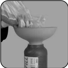
Put a funnel on the empty cartridge and fill in the new resin.
