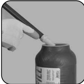
Clean threads from resin. Install filter head with O-ring seal and riser tube to cartridge.
